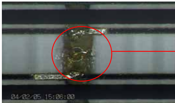
Panel electrode Insulation break down
